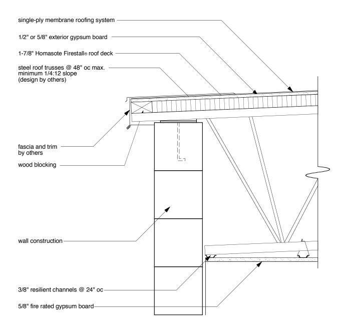
Firestall® Roof Deck Detail FS-SP-GBO-178-48-22 UL Design No. P535
