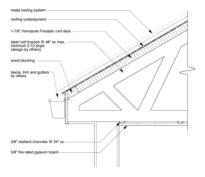
Firestall® Roof Deck Detail FS-MRD-178-48-19 UL Design No. P535
