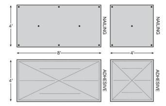
D. Wall Panel Installation: Space panel joints 1/8 inch (3 mm) apart; 1/4 inch (6 mm) space at floors, ceilings, and window and door frames. Install gypsum wallboard or other wall finish panels so that finish panel joints are staggered and do not coincide with sound barrier panel joints. Install in accordance with finish panel manufacturer's installation recommendations.
